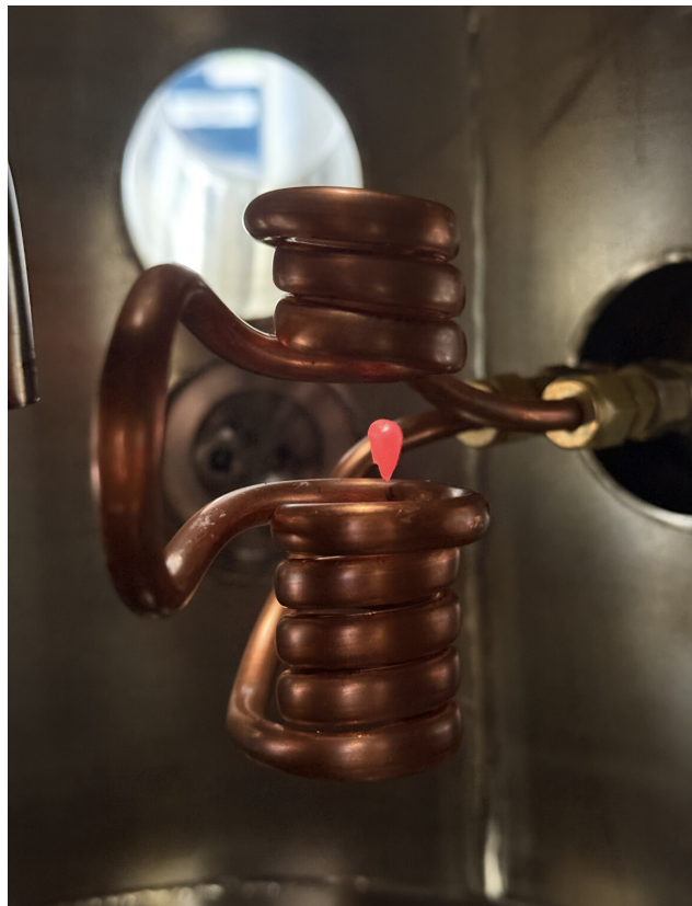
Figure 2.1 : Dramatic Sample Deformation Observed in Land-Based Electromagnetic Levitators
