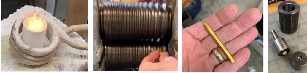
Figure 3.1 : Preparation of the Ingot Blank Showing Induction Melting, Ingot Rolling, Ingot Trimming and the Creation of the Press Fit Blank
